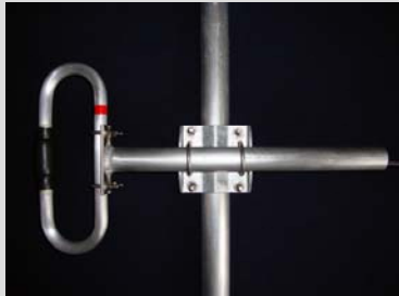
1/4 - wave spacing (9.4 – 9.7 dBd gain) (Offset pattern)
